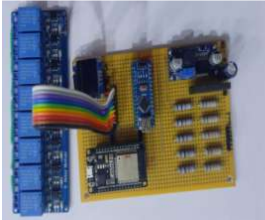
Fig.5 Controller of Charging Station
